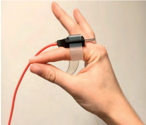
Figure 1. Accelerometer positioned at the base of the right index finger.
